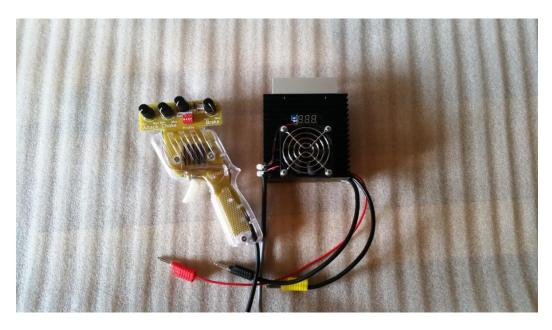
25 steps, all equal size. Trigger response can be adjusted using profile switches to make controller softer or more aggressive.
